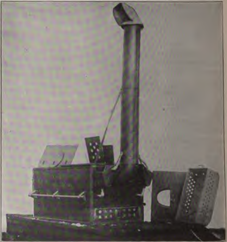
FIG. 224.—The Q. M. C. incinerator, No. 1, Model 1911. Showing urinals, cast-iron lid, wooden seat and charcoal burner.
